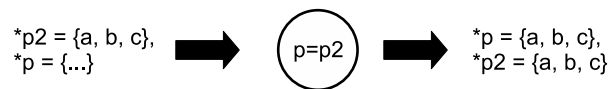
Figure 5.2: An assignment from one pointer to another will replace any previous mappings with a copy of the other pointer's mappings.
