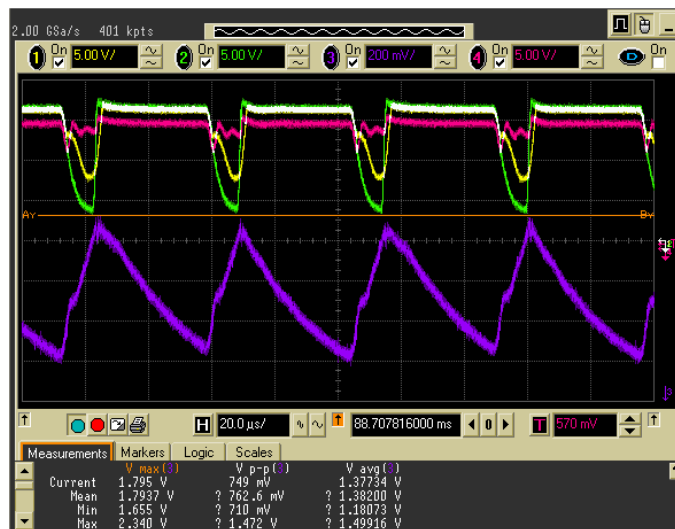
Figure 4.1: Waveforms of a BLDCm feed with PWM. The lower waveform is the measured phase current and the upper waveforms is the phase voltages
