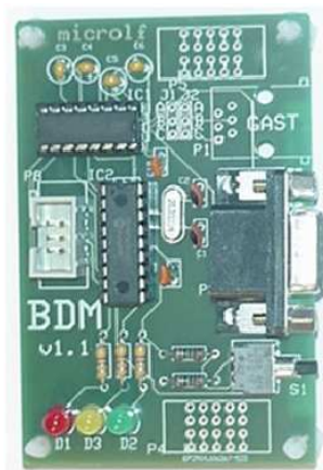
Figure 3.5: The GAST BDM hardware adapter used to update the software for the HCS12 controller.
